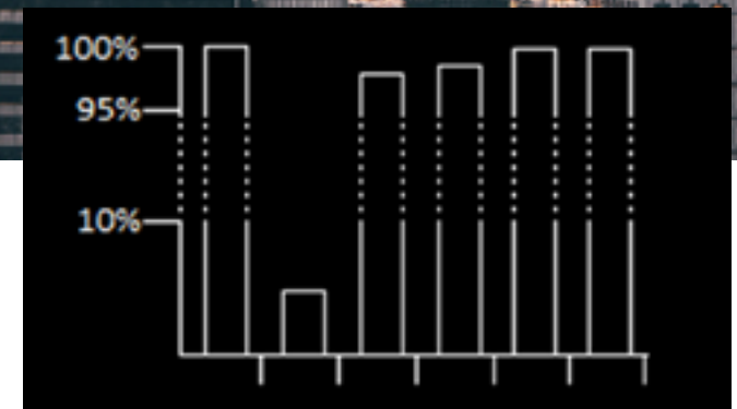
Fig. 4: Using dynamic breaks in data series with wide ranging values can save a lot of valuable display space
