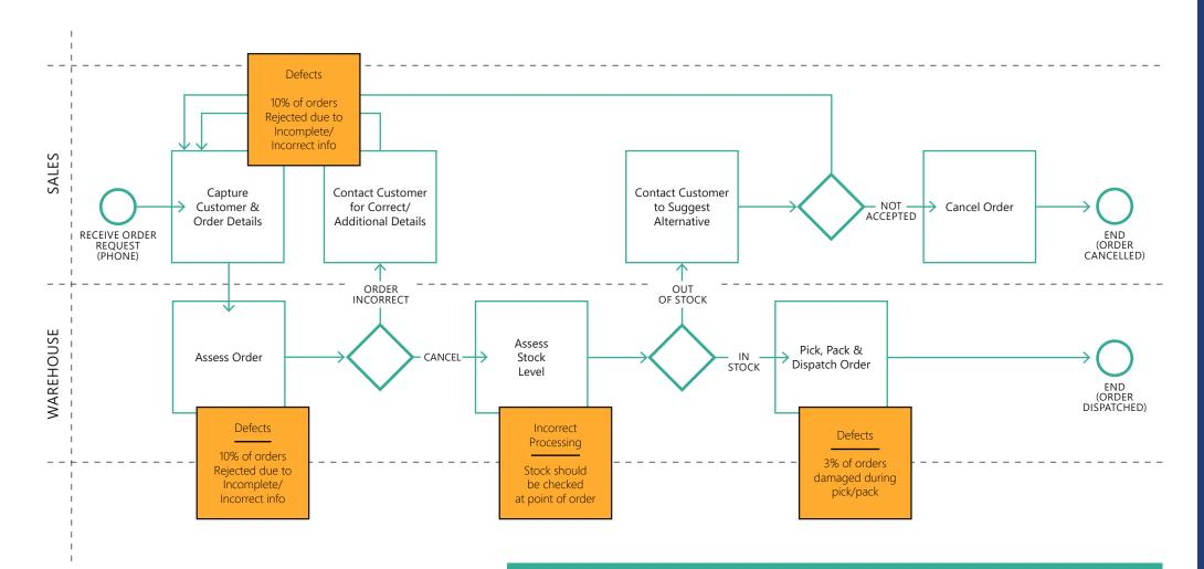
Figure 2: An initial informal sketch of a process, with some potential areas of waste highlighted
