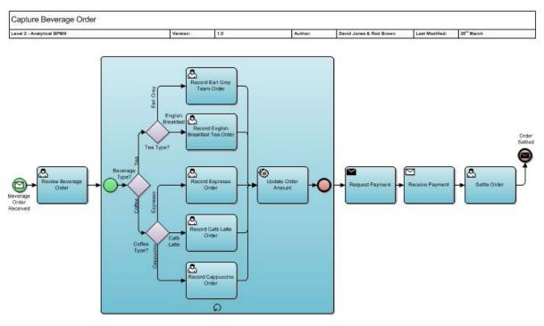
Figure 4: Example Process Diagram
