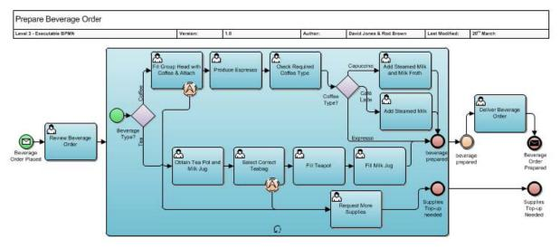
Figure 33: Process Diagram - Prepare Beverage order
